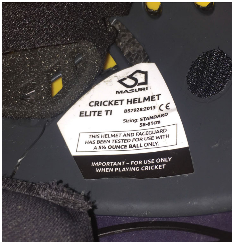
Figure 4: BS7928:2013 certification sticker on the inside of the helmet shell.
