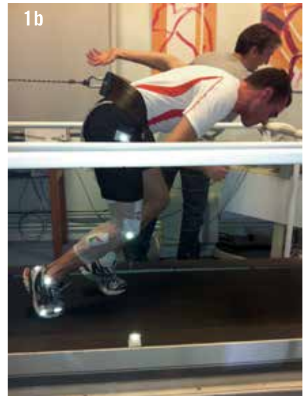
Figure 1: The instrumented sprint treadmill. Subjects are attached to a wall and can accelerate from a still crouched position. It is possible to synchronise electromyography measurements and video motion analysis. 1c) World-class sprinter Christophe Lemaitre sprinting on the treadmill.
